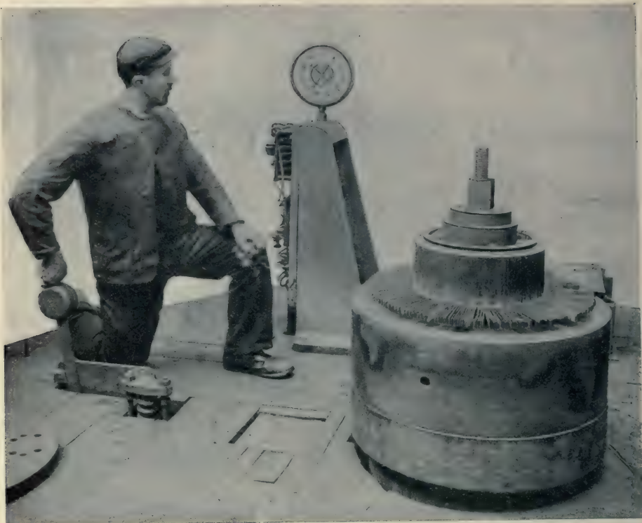
FIG. 132.—200-ton Press for squeezing Commutators. Vickers, Sons & Maxim.
